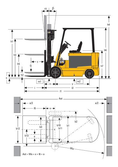
Ast = Working aisle width with load
