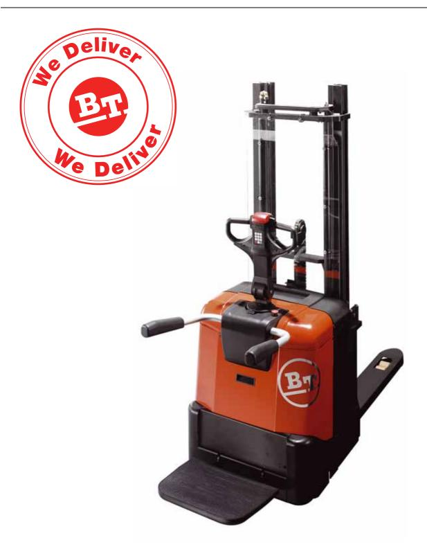
SPE125 and SPE160 both have fixed support arms and lift heights up to 5400 mm. The machines are built for horizontal transport and stacking in intensive applications that require durable high capacity trucks.
