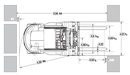
$$\begin{split} & \iota_{st} = \ Wa + x + I_6 + a \\ & \text{pplies only if} \quad \frac{b_{12}}{2} < b_{13} \\ & \iota_{st} = \ Wa + \sqrt{(\ I_6 + x)^2 + \left(\frac{b_{12}}{2} - b_{13}\right)^2} + a \\ & \text{pplies only if} \quad \frac{b_{12}}{2} \ge b_{13} \\ & = 200 \end{split}$$
