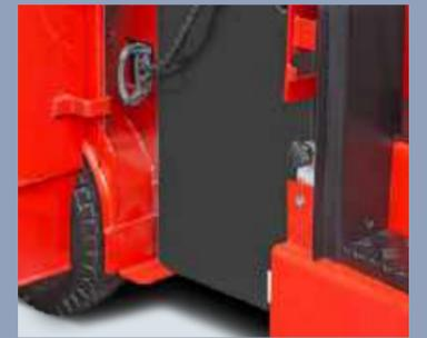
The battery can be removed from truck side, so it is very convenient for battery maintenance
