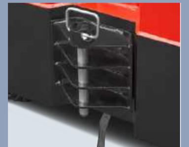
Upon special design, the traction device can prevent the towing pin coming off during traveling
