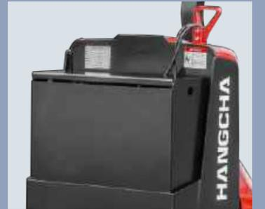
The battery compartment is sized to fit either a 12-85-5 industrial battery in its 7.8 inch compartment for heavier throughput applications
