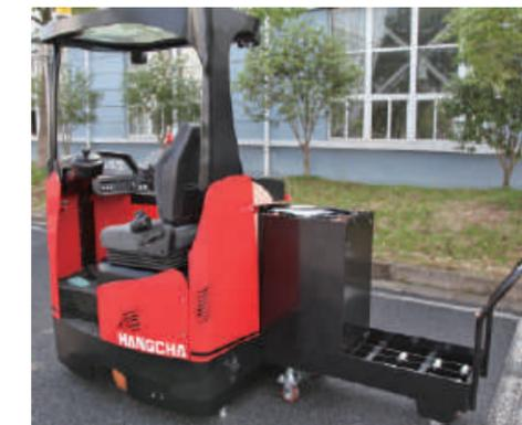
*Standard configuration: Battery side roll-out + trolley(optional)*
