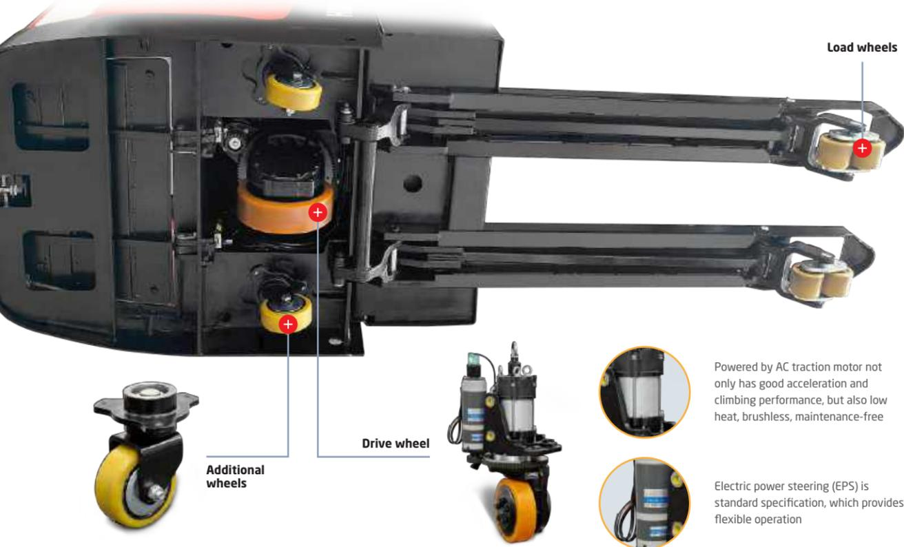
Powered by AC traction motor not only has good acceleration and climbing performance, but also low heat, brushless, maintenance-free
