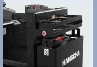
The rear load tray can be folded for working in confined space
