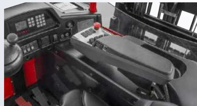
Whichever of above two modes the operator wants to select, there has a button for switching operation to activate the mode required, which can be selected freely by the operator according to his/her habit. The electric steering wheel is small and light. The operator can adjust it by moving backward or forward to find a suitable position. The steering wheel have built-in damper, with reliable signal transmission of stepping motor.
