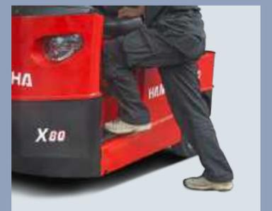
Low-level widely open foot board is very convenient for the operator to get on / off the truck
