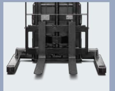
Fixed Straddle Baselegs ( Inside Dimension in 4" increments from 38" to 50"); Adjustable baseleg optional to fit a wide range of pallet sizes
