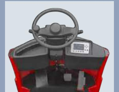
Various operating pedals, instruments, steering wheel, and switches are configured based on ergonomic requirements, and are comfortable and flexible for operation
