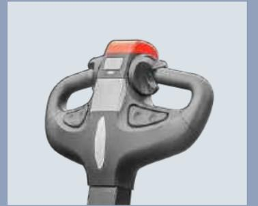
Simple and beautiful tiller designed to operate all functions easily even by one hand. Displayed turtle speed function applied to move slowly and helps to stack goods in narrow spaces
