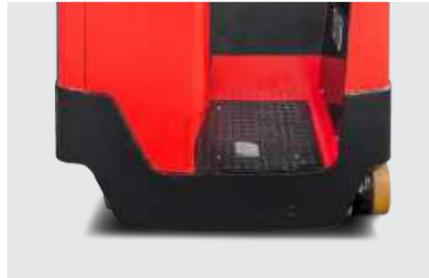
The low pedal enable the operator to get on and off the truck more conveniently and comfortably.
