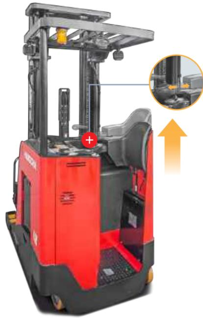
The control handle and backrest can be adjusted according to the operator's habits.
