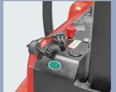
Built-in charger and maintenance free gel battery adopted to provide convenient usage
