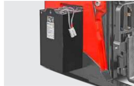
The lateral removal of the battery provides easier maintenance and is applicable to continuous operating conditions.
