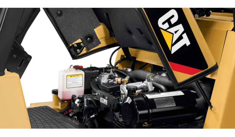
With a smooth running GM 4.3 liter V6 engine, powerful transmission and dependable cooling system, these LP Gas cushion tire lift trucks will get the job done.
