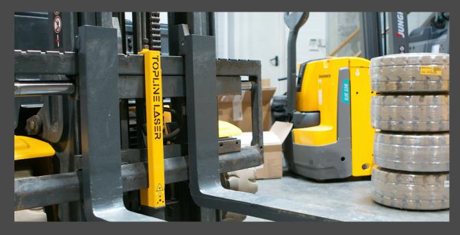
The TOPLINE LASER attachment can be especially useful when working with irregularly shaped or oversized loads as it can help the forklift operator accurately position the forks and avoid damage to the load or surrounding objects. It can also improve efficiency by reducing the time required for each lift, as the operator can quickly and accurately position the forklift without the need for multiple adjustments.
